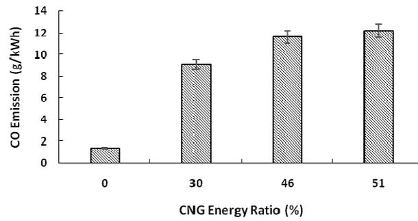
Figure 5: Comparison of CO Emission with CNG Share
