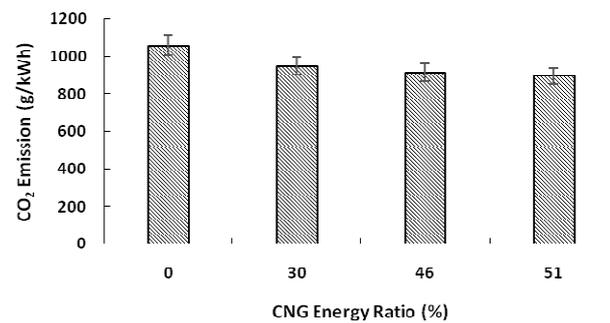
Figure 6: Comparison of CO<sub>2</sub> Emission with CNG Share
