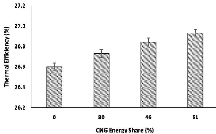
**Figure 4: Comparison of BTE with CNG Share**
