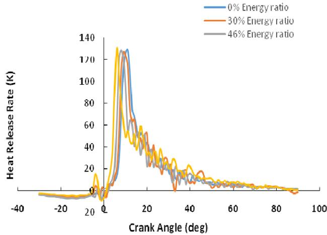
**Figure 3: Comparison of Heat Release Rate with Crank Angle & CNG Share**
