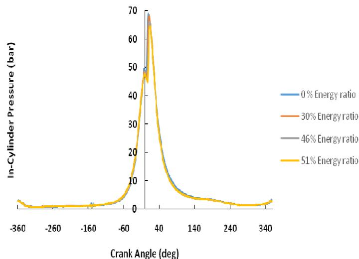
**Figure 2: Comparison of In-Cylinder Pressure with Crank Angle & CNG Share**
