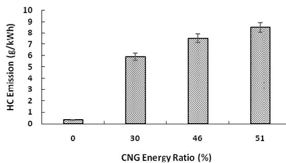
Figure 7: Comparison of HC Emission with CNG Share
