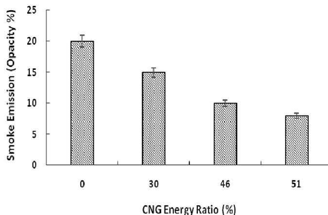
Figure 9: Comparison of Smoke Emission with CNG Share
