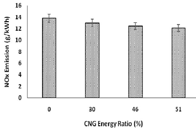
Figure 8: Comparison of NO<sub>x</sub> Emission with CNG Share
